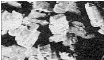
Heavy zinc phosphate crystals break off easily when handled, leaving exposed bare areas between the crystal roots to corrode. The coating has poor adhesion and the excess material causes galling.
